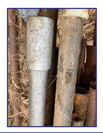
What we see here on the right, is a picture of tubing that's been in the hole for 8-12 months. They had to pull the tubing because of hole in it from corrosion. That's common that they only get 8-12 months out of their tubing.
